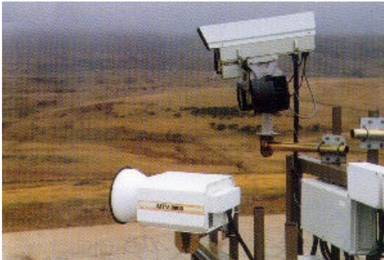
Two microwave transmitters
